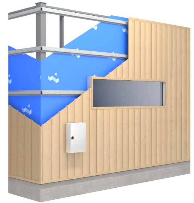
Cladding - Vertical Over Top Hats View Alteria's Cladding Installation Guide for details.
