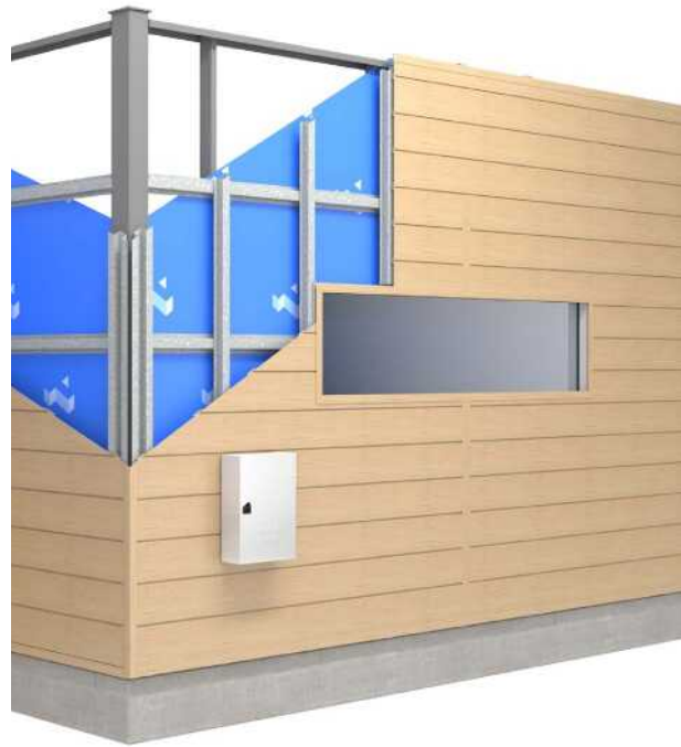
Cladding - Horizontal Over Top Hats Go to page 18 for installation details.
