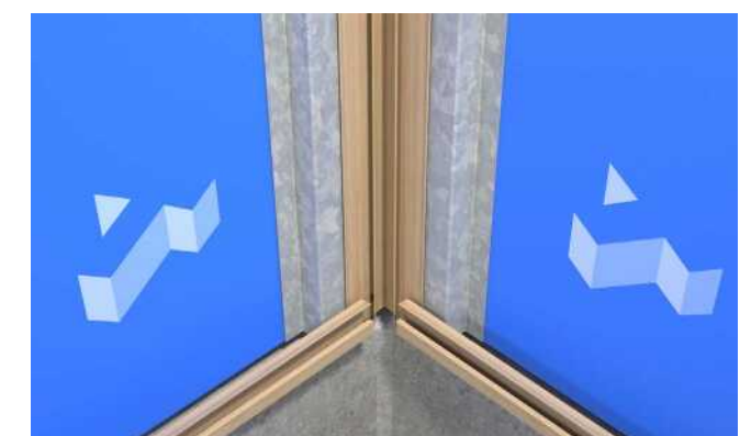
Step 2. Screw the Starter Profile to the bottom of the corner.
