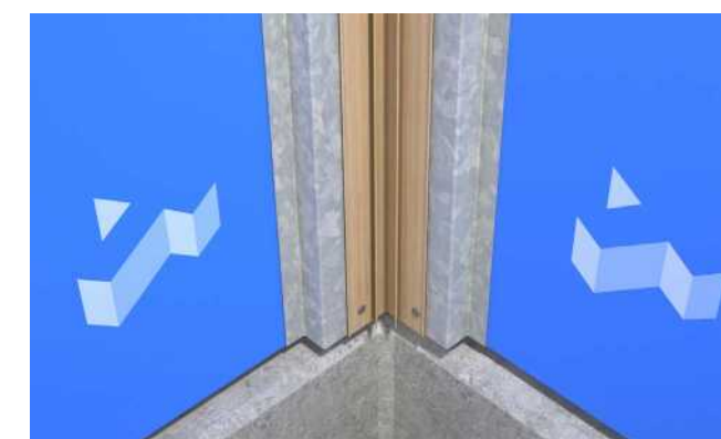
Step 1. Screw the Female Corner Profile to both sides of the corner structure. Note: Ensure screws have sufficient clearance to not interfere with Starter Profile.
