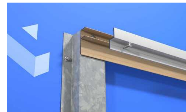
Step 1. Screw the Female Finisher Profile to the centre of the top hat or structure then screw Z Support Profile below the Female Finisher Profile.
