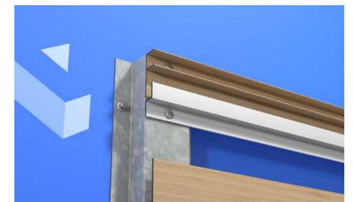
Step 2. Place the cut to size cladding board on top of the Z Support Profile, and just underneath the inside leg of the Finisher Profile. Secure board into place.
