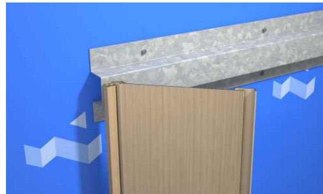
Step 2. Insert vertical cladding board into the Starter Profile.
