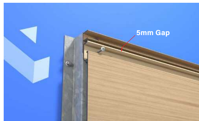
Step 2. Place full size cladding board on top of the Male Finisher Profile and secure with screws. Ensure to leave a 5mm gap between the trim piece cladding board.
